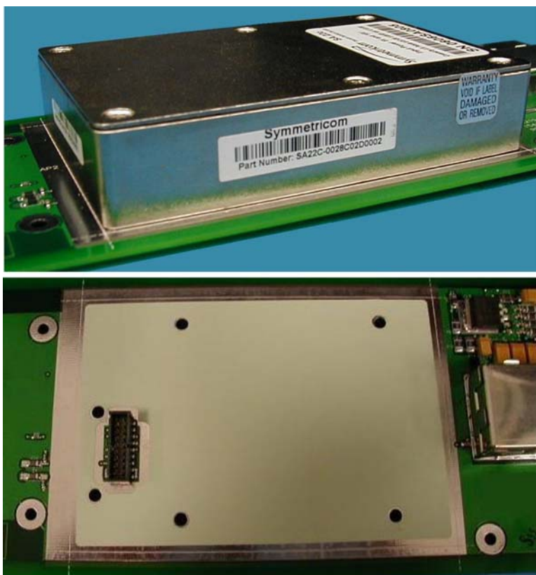
Figure 2-1. Mounting an SA.22c to a Circuit Board
